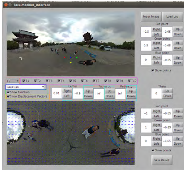
Figure 20: in red: current transformation pop-up button; in blue: smoothing function pop-up button; in green: Show function box; in yellow: show displacement vectors box; in pink: T_i boxes; in orange: Center coordinates of smoothing function, R_x, R_y and \theta , respectively; in cyan: Right, Left, Up and Down buttons.
