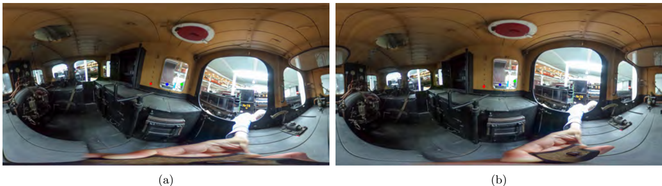
Figure 6: An example of elliptic Moebius Transformation. (6b) the result of a rotation by 10^\circ degrees ( T : [(-0.3 \ 0), (0 \ 0), (0.3 \ 0)] \rightarrow [(-0.2954 \ -0.0521), (0 \ 0), (0.2954 \ 0.0521)] ).
