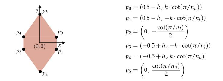
So, the coordinates  $p_0, \ldots, p_5$  depend on the parameters  $h, n_u$ , and  $n_l$ .
