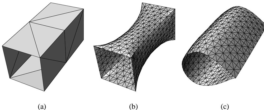
Fig. 11. Control of shape features and boundary treatment: (a) initial mesh; (b) tagged boundary edges; (c) tagged internal edge.
