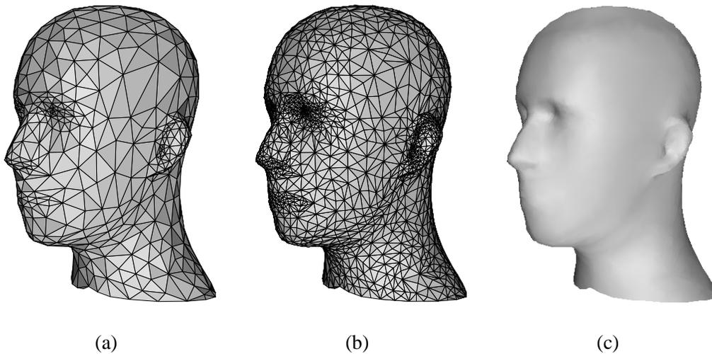
Fig. 10. Mannequin head. Control mesh (a), two levels of subdivision (b), Flat shading after nine levels of subdivision (c).
