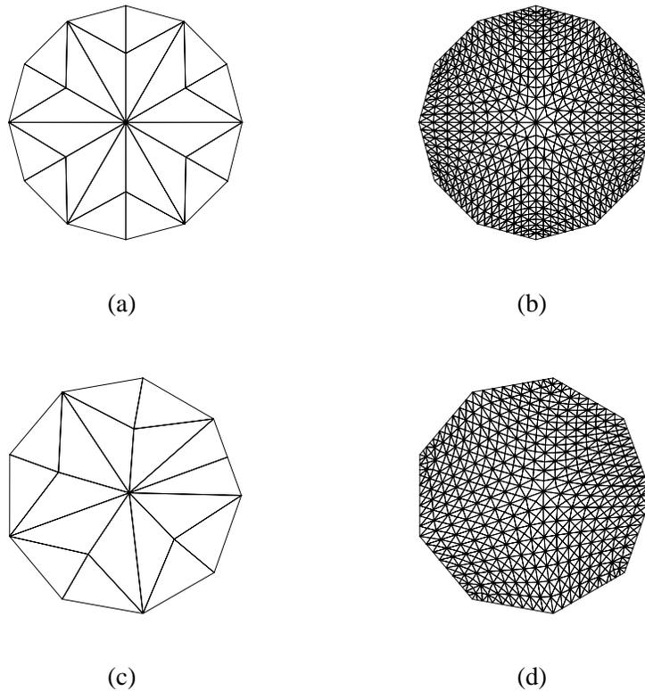
Fig. 8. Subdivision of regular polygons with even (a,b) and odd (c,d) number of sides.
