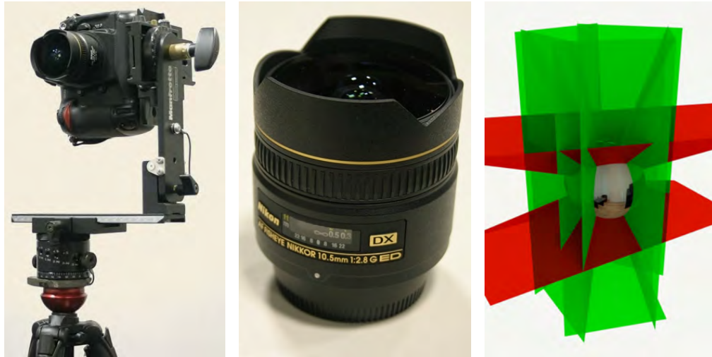
(a) Manfrotto Pano Head, Nikon DX2S camera and Nikon 10.5mm fisheye lens.
