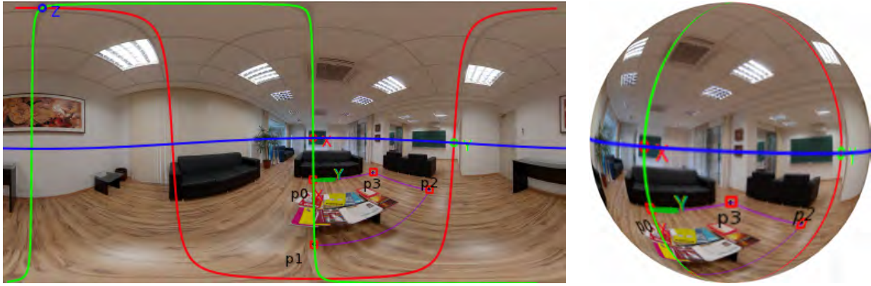
Figure 3: Left: Panorama alignment system. The four points on the floor determine the orientation axis for the environment. The blue, red and green lines illustrate the xy (horizon), xz and yz slice planes respectively. Right: Spherical representation of the panorama with the axis.
