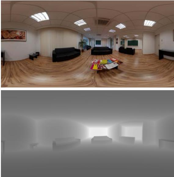
Figure 2: The upper picture shows the radiance channel of the environment and the lower one the depth channel used for reconstruct the light positions.
