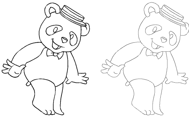
Figure 2. The skeletonization of the figure on left removes extra pixels and produces a simpler image (right).
