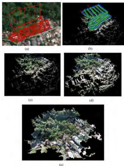
Fig. 3. BOC 60 Steps to Rebuild PIX4D software; (a) Snapshot points on the map; (b) 3D image taking points; (c) Tie Points; (d) Dense cloud of points; (e) Textured 3D Model.
