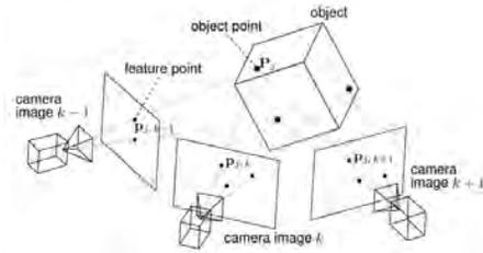
Fig. 2. Result after structure-from-motion estimation. The projection of a 3D object point  $P_j$  in the camera image at time  $k$  gives the tracked 2D feature point  $P_{j,k}$  [2]
