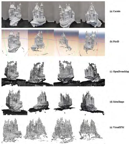
Fig. 6. Medieval Castle experiment, reconstruction using different tools.
