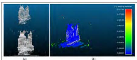
Fig. 7. Comparison point cloud Metashape and OpenDroneMap, Metashape reference. (a) Insertpoint cloud, Metashape cloud top, and OpenDroneMap cloud bottom; (b) Generated heat map.
