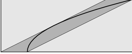
Figure 3: Zonotope approximation of a parabola segment.
