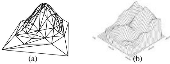
Figure 2 – TIN (a) and Grid representation (b) of
