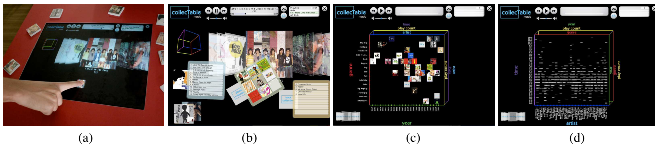
Figure 1: The collecTable running on the iTable (a), with several fiducials over it. The digital projections of the fiducials floating over the interface (b), each fiducial storing different music collections. The M-Cube interface for music data showing albums (c) and tracks (d).
