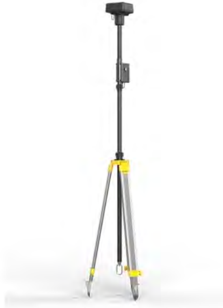
Figure 21 – RTK base station with GNSS antenna, radio modem and power module; used to provide differential corrections to airborne RTK receivers. Source: From (3)
