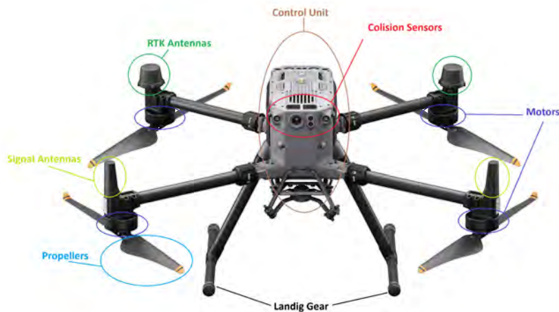
Figure 19 – DJI Matrice 350 RTK — annotated external components: propellers and motors, collision sensors, landing gear, battery compartments and RTK antennas. Source: Adapted from (3)
