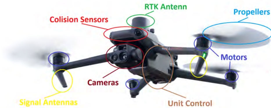
Figure 18 – DJI Mavic 3T Enterprise — annotated external components: propellers and motors, collision sensors, landing gear, battery compartments and RTK antenna. Source: Adapted from (3)
