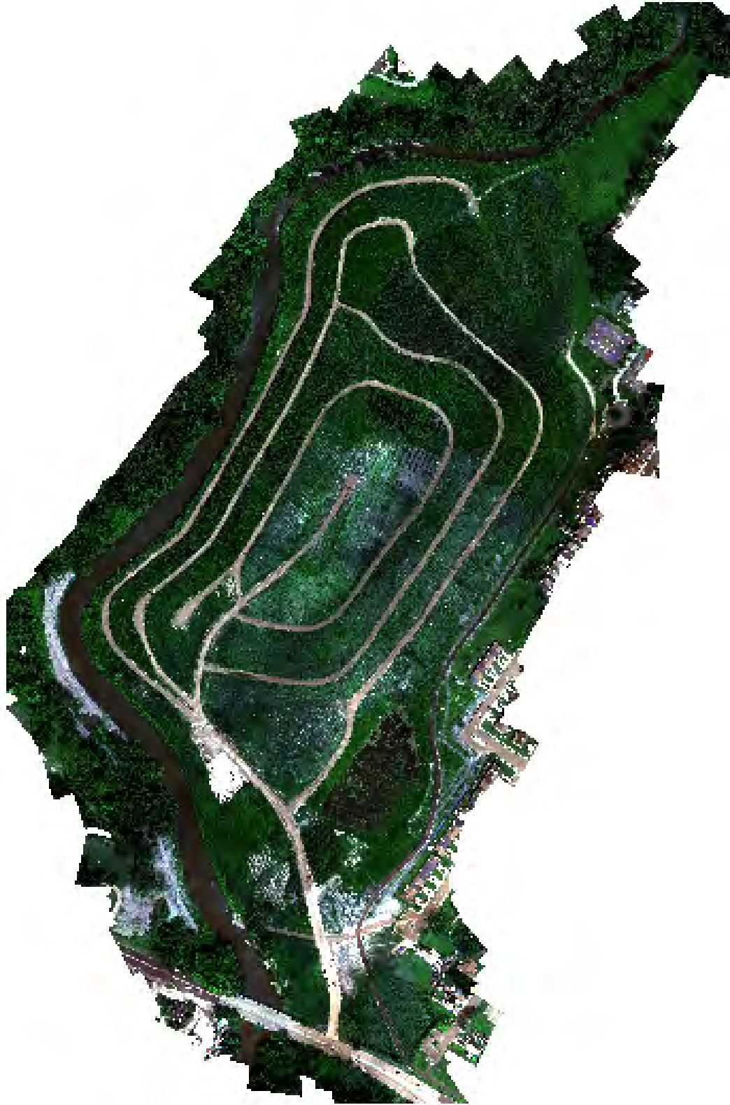
Figure 39 – Overview of the USGS Darby dataset, integrating LiDAR cloud, RGB bands and thermal layer. Source: From (5)
