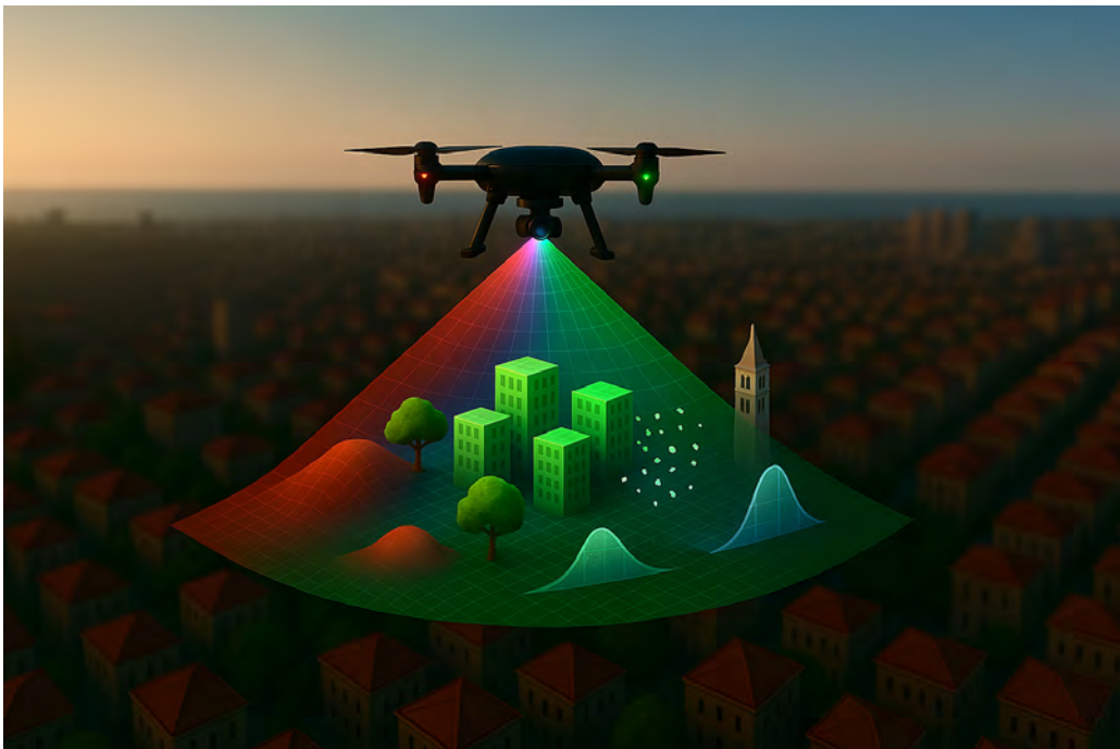
Figure 1 – Conceptual illustration of multimodal UAV acquisition and processing. The colored cone represents the sensor coverage integrating RGB, thermal and LiDAR channels, which can be combined in a integration and continuous rendering pipeline. Illustrative parameters: typical flight altitude 40–80 m; field of view and cone shape depend on payload and mission profile.
