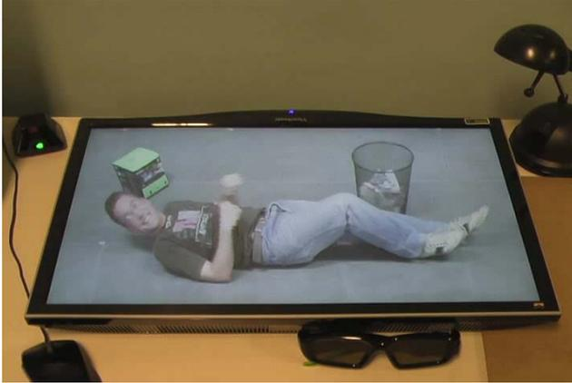
Figure 11. The Virtual Table is showing an image whose scale was chosen in such a way that the quadrilateral border generated after applying the homography is outside the display.
