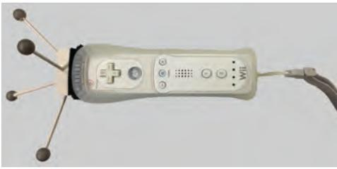
Fig. 4. Wand based on Wii mote.
