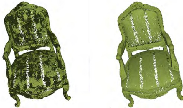
FIGURE 5. Visualization of surfels (bright means the normal is facing the camera, dark otherwise) of results of back-face culling. On the left, we have no back-face culling; on the right, we add back-face culling. Green means the surfel points to the camera, and black means otherwise. As seen in this image, adding back-face culling forced the surfels to be consistently aligned, as expected.
