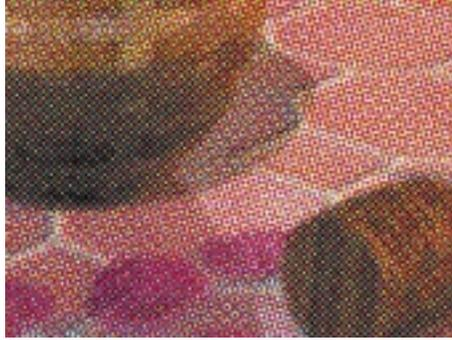
Figure 5: Detail of the printed *CMYK* channels from Figure 1.
