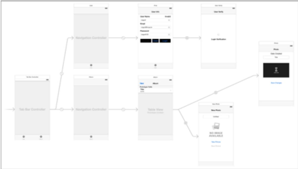
Each view has a controller class which contains the functionality of UI elements. On the top branch there is a path which leads to the login and authentication UI. The lower path leads to the server picture list and through buttons such as New or Edit, it is possible to navigate to the Camera View and Picture View.
