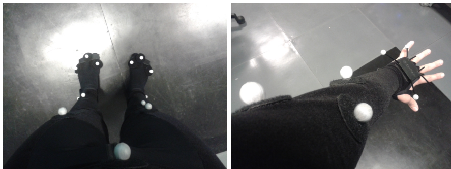
FIGURE 3 – Retroreflective sensors placed on a performer
