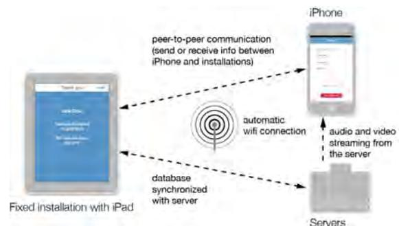
**Figure 2:** Expo Framework exploits different communication mechanisms for content interaction.
