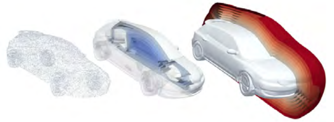
Fig. 10. The level sets of an MLP trained with the IGR method on an input point cloud; positive level sets are in red; negative are in blue; the zero level set, representing the approximated surface, is in white.
