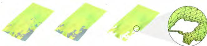
Fig. 9. Topology repair operator. Left to right: original mesh, after *hole texture* edition, and final mesh.
