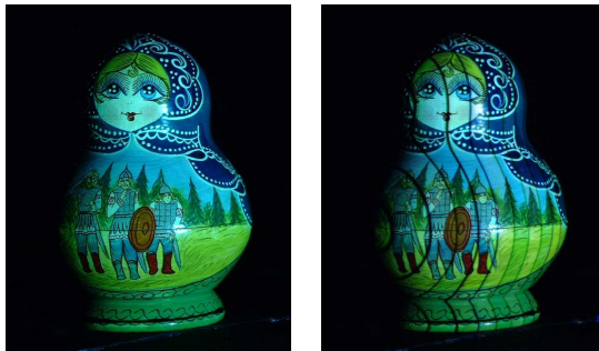
(b) Object illuminated with real white light (left) compared to the recovered white light from processing a pair of complementary slides (right).
