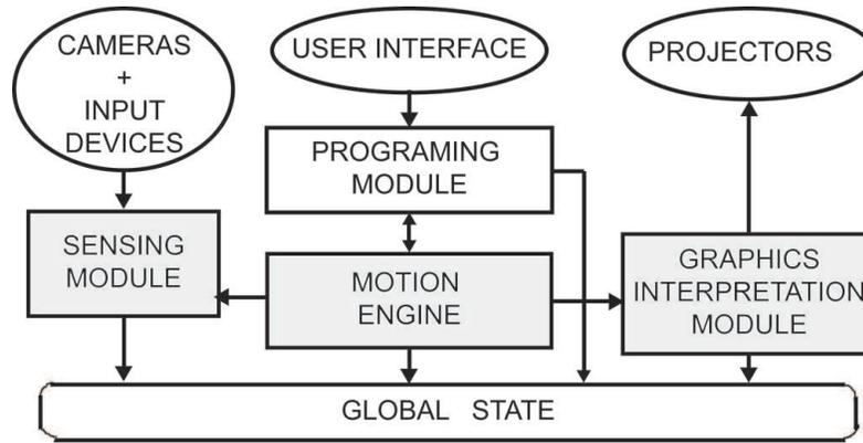
Figure 1: X-Motion System Architecture.
