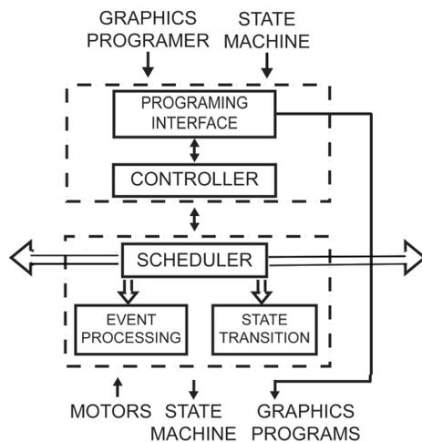
Figure 4: Motion Engine and Programming Module.
