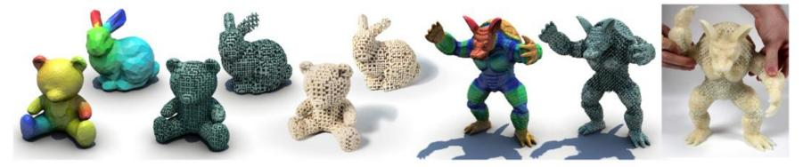
Figure 1: Given a virtual object with specified elasticity material parameters (blue=soft, red=stiff), our method computes an assemblage of small-scale structures that approximates the desired elastic behavior and requires only a single material for fabrication.
