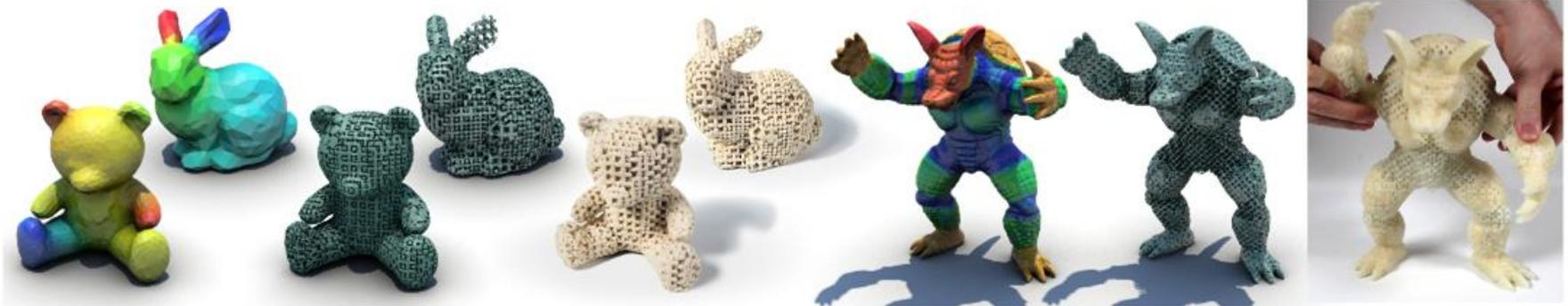
**Figure 1:** Given a virtual object with specified elasticity material parameters (blue=soft, red=stiff), our method computes an assemblage of small-scale structures that approximates the desired elastic behavior and requires only a single material for fabrication.
