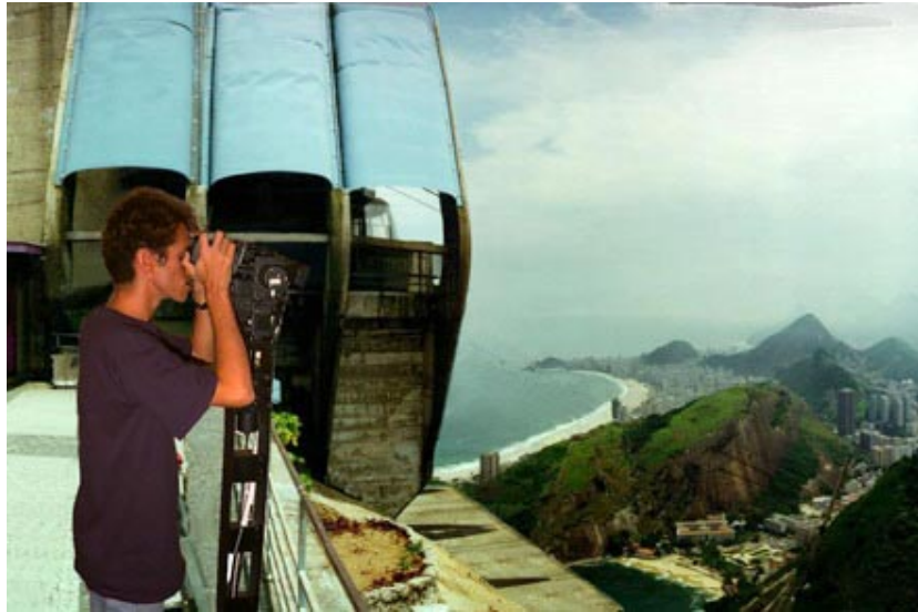
Figure 2. The Visorama prototype installed in a tourist site. The user is looking at a panorama created from the same location and edited to show the surroundings at different times in history.
